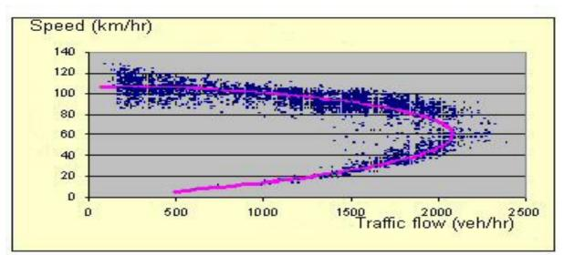
Figure 4. The relationship between traffic flow and speed for an urban motorway.
