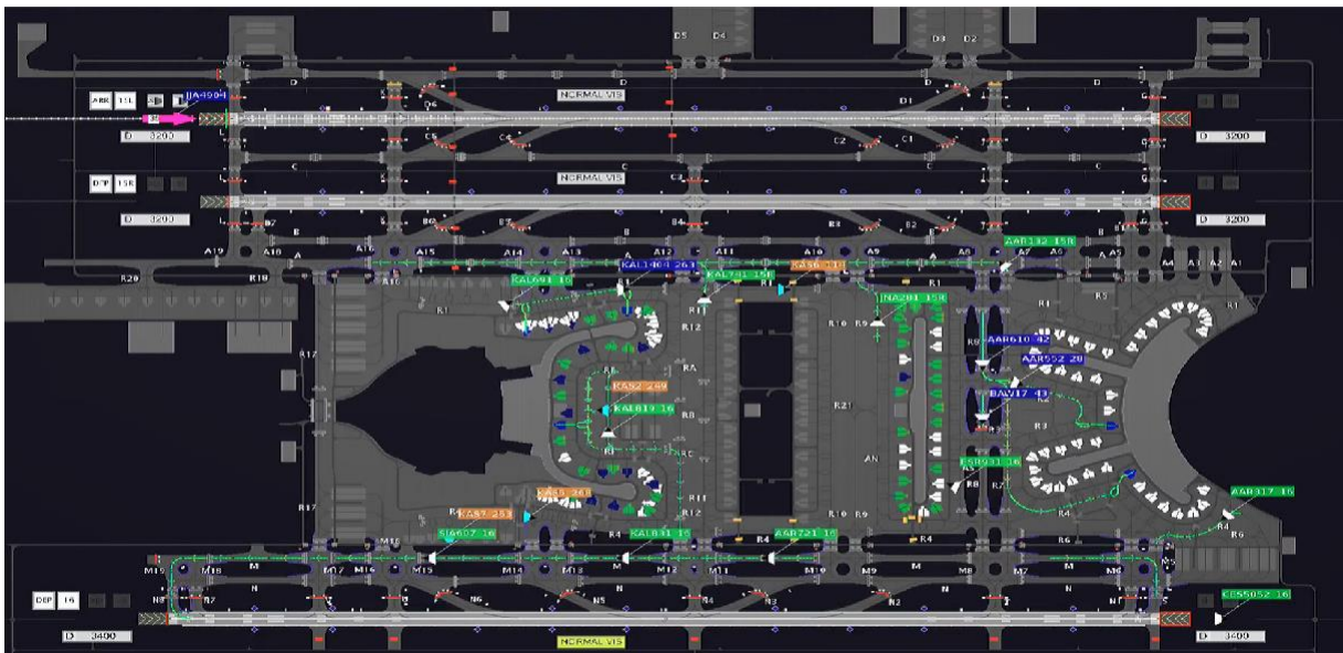
Figure 13. Dashboard of a surface movement control system at Incheon International Airport
