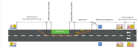
Figure 17: Closure of the Right-Hand Lane of a Multilane Carriageway
