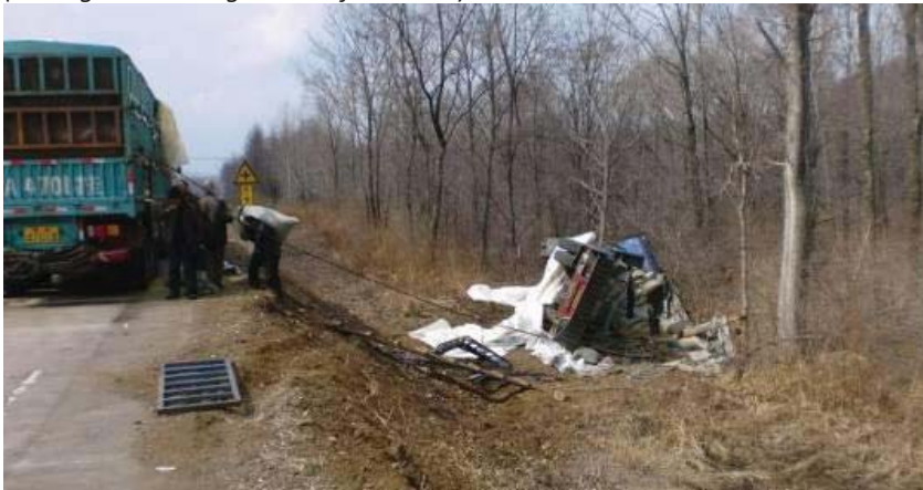
FIGURE 4.2.2.4 ROLLOVER OF A TRUCK ON 1:1.5 EMBANKMENT SIDE SLOPE (driving is on the right side of the road)
