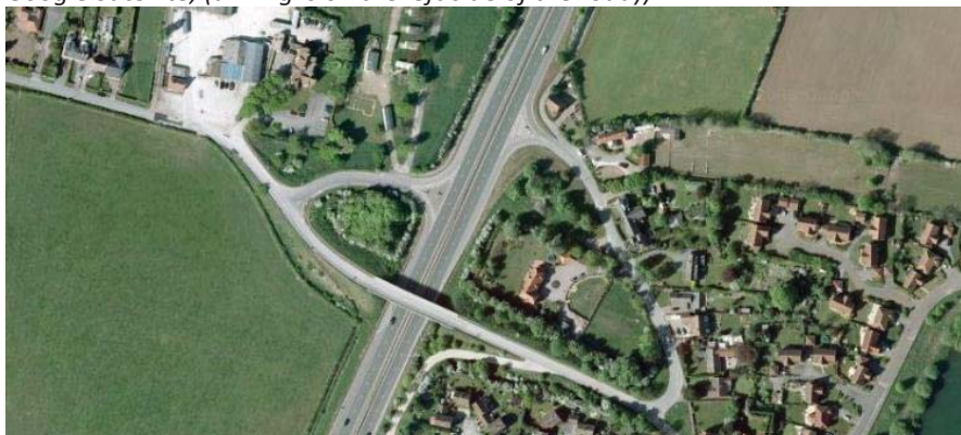
FIGURE 3.6.3.1 COMPACT GRADE INTERSECTION INTEGRATED INTO THE LOCAL ROAD NETWORK (ref: Google Satellite, (driving is on the left side of the road))
