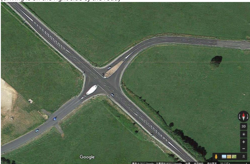
FIGURE 3.2.3.2 SIDE ROAD CHANNELIZING ISLANDS AT A CROSSROAD INTERSECTION (driving is on the right side of the road)
