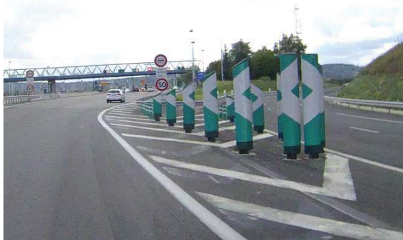
FIGURE 6.2.2.6 DELINEATORS AT DIVERGE GORES (driving is on the right side of the road)
