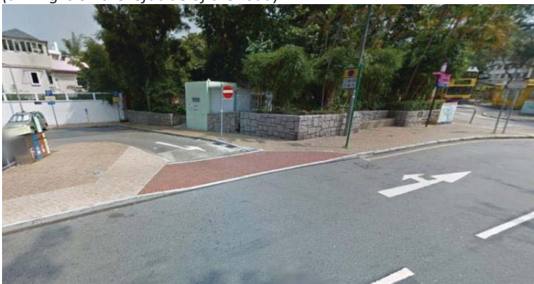
FIGURE 5.2.2.4 COLOUR CONTRAST AT A DIRECT FRONTAGE ACCESS (driving is on the left side of the road)
