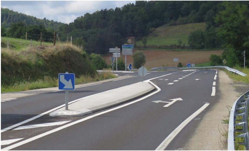
FIGURE 3.2.5.4 EARLY TERMINATION OF PHYSICAL TRAFFIC ISLAND (driving is on the right side of the road)
