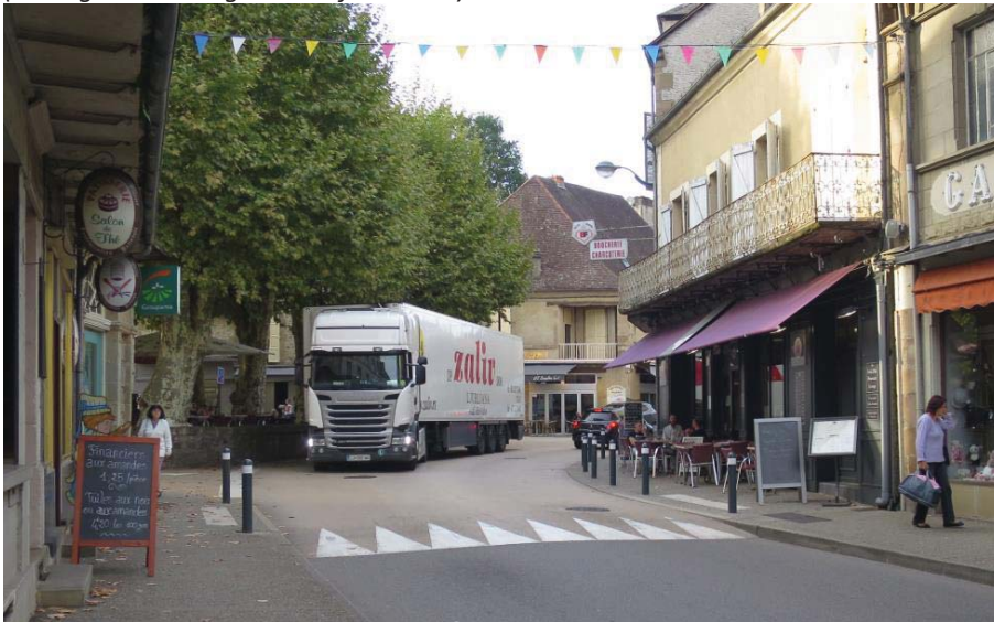
FIGURE 5.4.3.2 SPEED TABLE AT THE CORE AREA OF AN URBANISED SECTION (driving is on the right side of the road)
