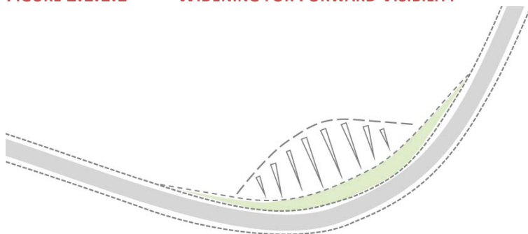
FIGURE 2.1.1.1 WIDENING FOR FORWARD VISIBILITY
