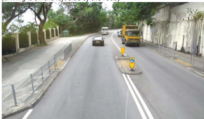
FIGURE 5.2.5.4 HIGH VISIBILITY PEDESTRIAN FENCE AT A CROSSING (driving is on the left side of the road)
