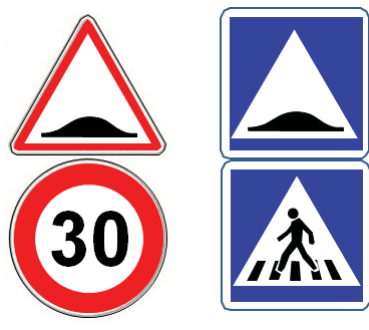
FIGURE 5.4.3.5 TYPICAL SIGNING FOR VERTICAL SPEED REDUCTION FACILITIES
