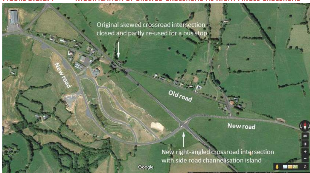
FIGURE 3.2.1.4 MODIFICATION OF SKEWED CROSSROAD AS RIGHT ANGLE CROSSROAD
