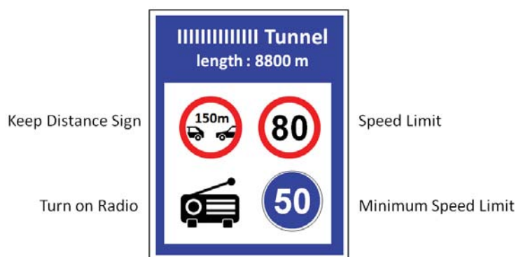
FIGURE 8.3.1.1 POSSIBLE SIGN DISPLAY CONTAINING ESSENTIAL INFORMATION
