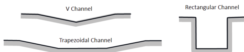
FIGURE 4.2.3.1 COMMON TYPES OF OPEN DITCHES
