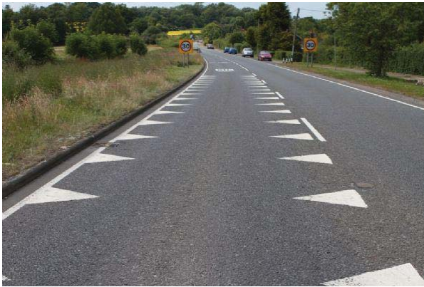
FIGURE 5.4.2.6 OPTICAL SPEED BARS (ref: FHWA, US, driving is on the right side of the road)
