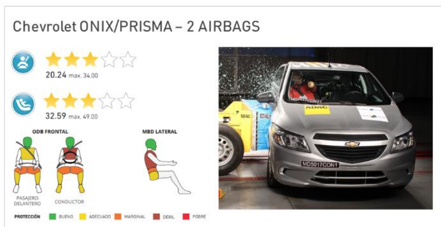
Figure 5. Chevrolet Onix/Prisma test result
