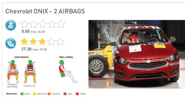
Figure 4. Chevrolet Onix test result
